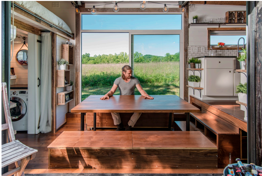
This tiny house boasts a large eating table and rolling benches that stow away completely underneath a raised floor when not in use. When open, this setup can accommodate eight people. (Designed and built by New Frontier Tiny Homes. Photograph by StudioBuell Photography.)
