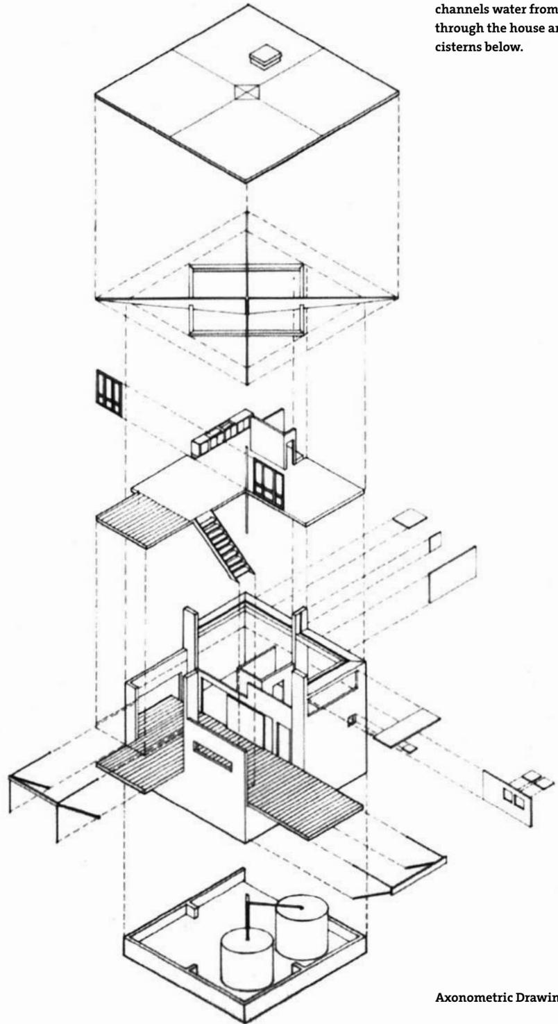
← The rain collection system channels water from the roof through the house and into cisterns below.
