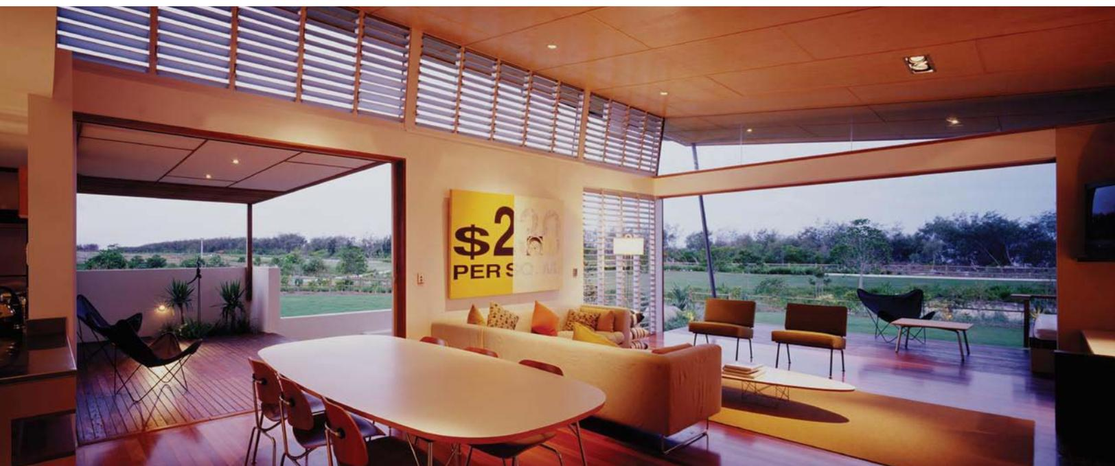
↑↑ The covered breezeway joining the two pavilions functions as a thermal chimney, coaxing hot air up and out while drawing in cool air from below.
