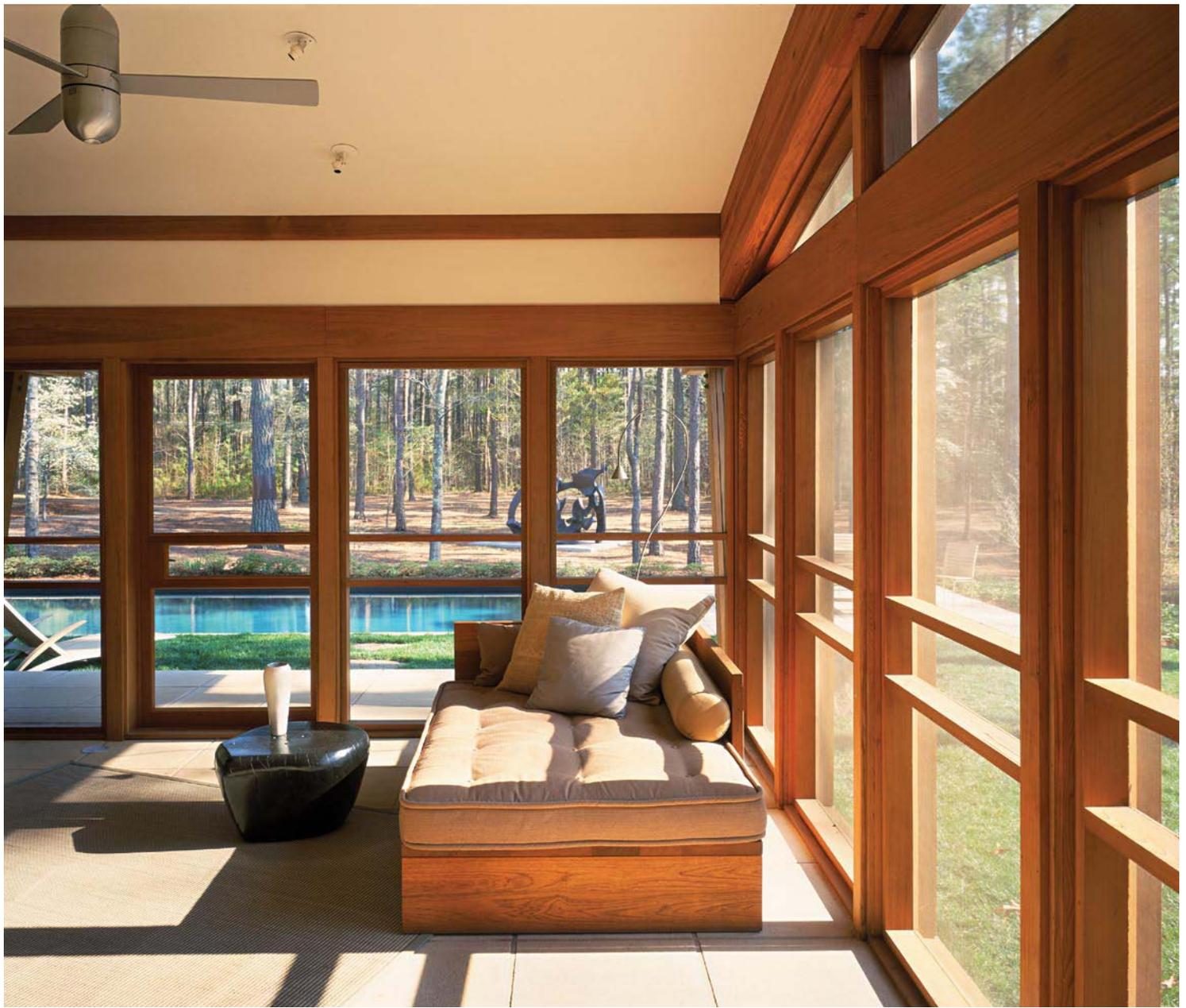
↑ The view of the surrounding woods is accentuated by large, gridded windows. Sunlight floods the interior during the winter, when the sun is low enough to slip beneath the exterior overhangs.
