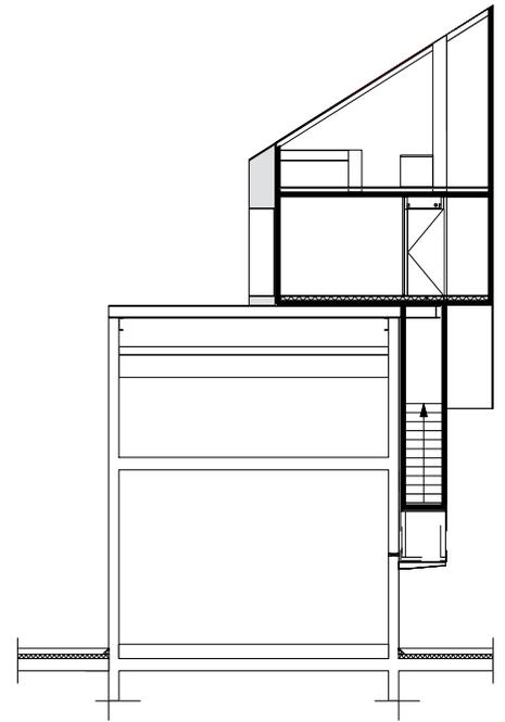
↖ | ↑ Elevations illustrate how the house perches atop the existing building's stairwell.
