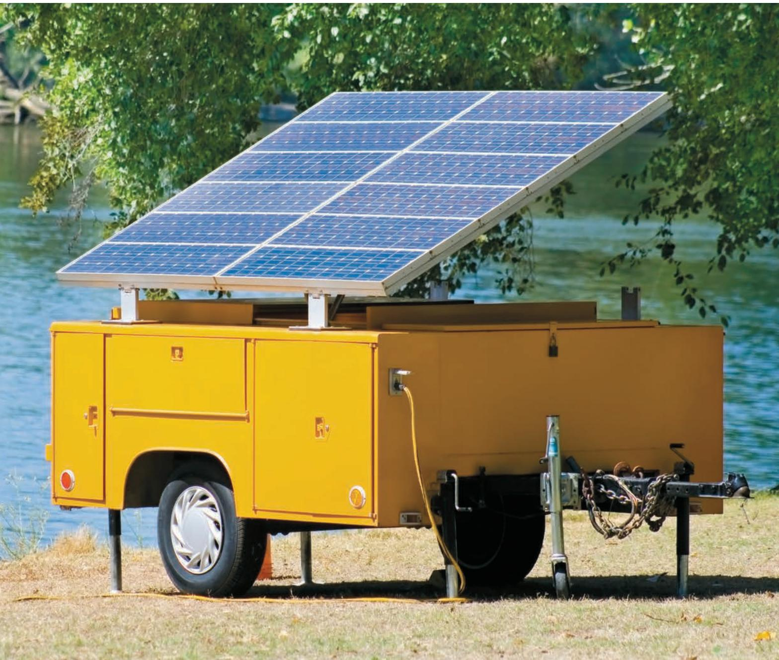
Solar trailers are commonly used for construction, disaster relief, outdoor events, and all kinds of work in remote locations. Enclosed trailers may include extra space for tool and equipment storage as well as a small office space.
