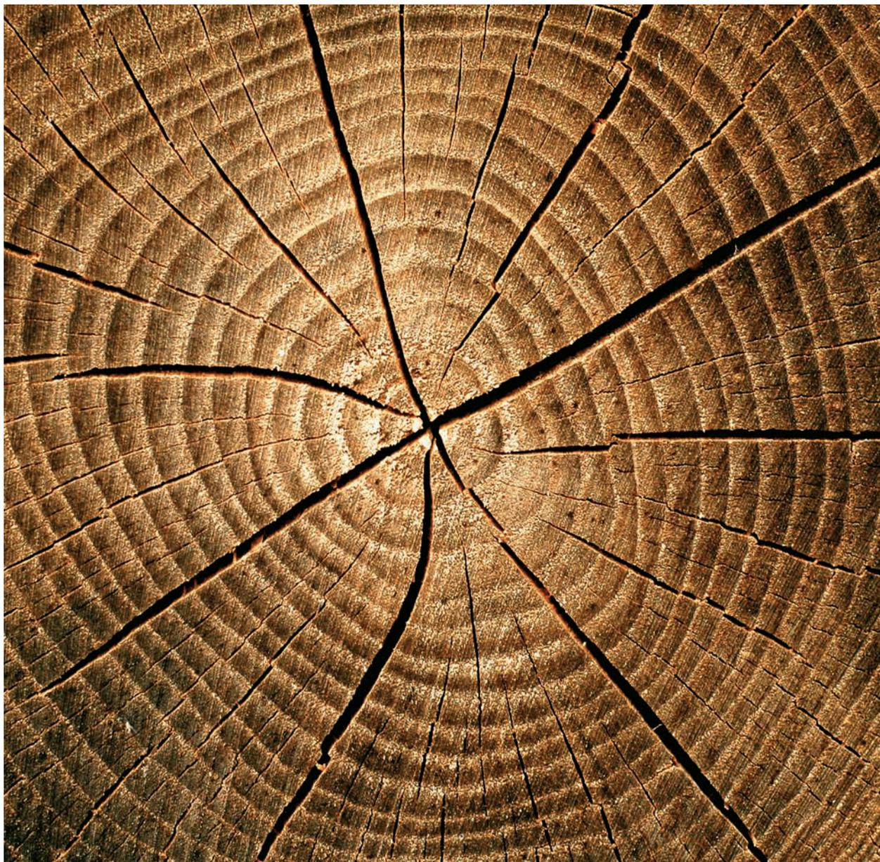
Up to half the weight of a freshly cut tree may be water, and as this water evaporates the wood shrinks, cracks, and warps. Controlled drying of wood can minimize these problems and produce a larger number of solid, furniture-grade boards.
