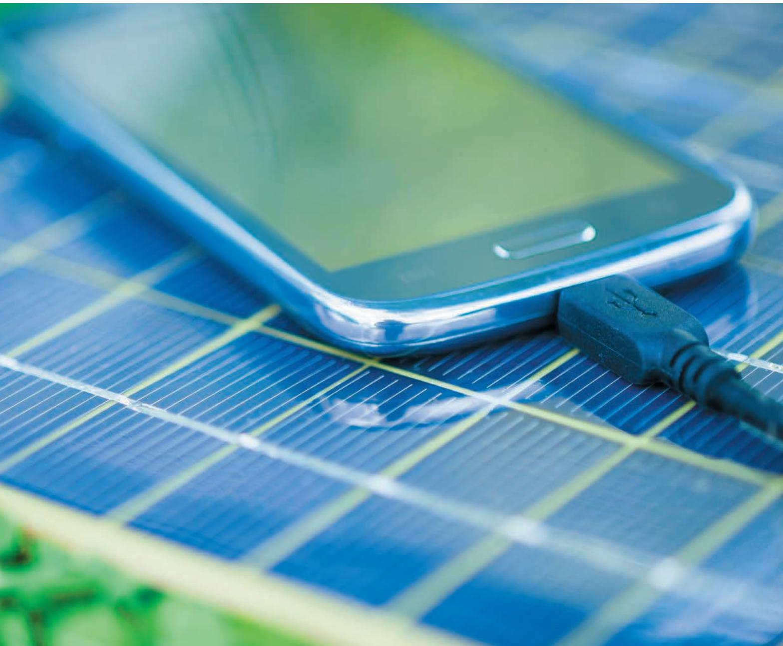
Cell phone chargers are small and lightweight, and generally produce 5 watts or less of power. A basic solar module such as this doesn't store power—it will only charge the cell phone when the sun is out.
