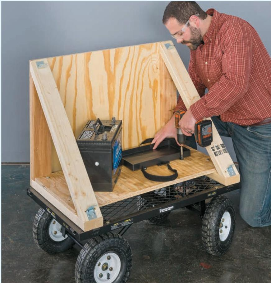
**4** Install the module mounting brackets onto the support legs, using 1½" screws, then test-fit the module. *NOTE: Leave the module covered with a tarp for safety; it will produce power even when exposed to artificial light. Determine the positions of the system components, including the battery, and mark the locations of holes for wiring runs through the plywood back panel. Also drill a hole through the base panel for a bonding wire between the bus bar and the cart bed.*
