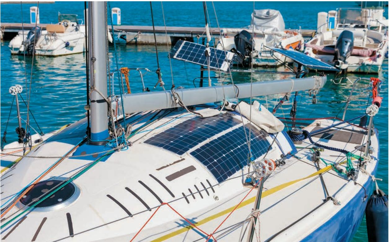
Flexible modules are thin and lightweight, in addition to being flexible, so they can go where rigid panels can't. Most flexible units have a grommet at each corner for easy tie-down.
