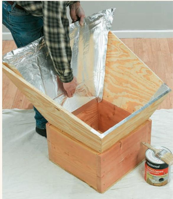
**11** Glue the reflective sheeting inside the base and reflector, overlapping the corners so all bare wood is covered. Use contact cement or silicone caulk to adhere solar foil, and staple the edges to reinforce the glue; use diluted white glue with a paint brush instead of contact cement if you're using aluminum foil. Pull or smooth out the reflective material as much as possible; the smoother the surface is, the better it will reflect light.
