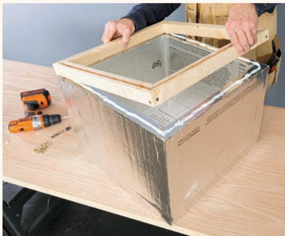
**3** Complete the box by cutting four pieces of  $2 \times 2$  channel to length at  $19$ ", mitering the ends at  $45^\circ$ . Glue the pieces to the top edges of the box sides with foamboard adhesive so all of the beveled grooves angle outward from the box center and they meet at the corners. Let the adhesive cure, then paint the interior of the box with black spray paint.
