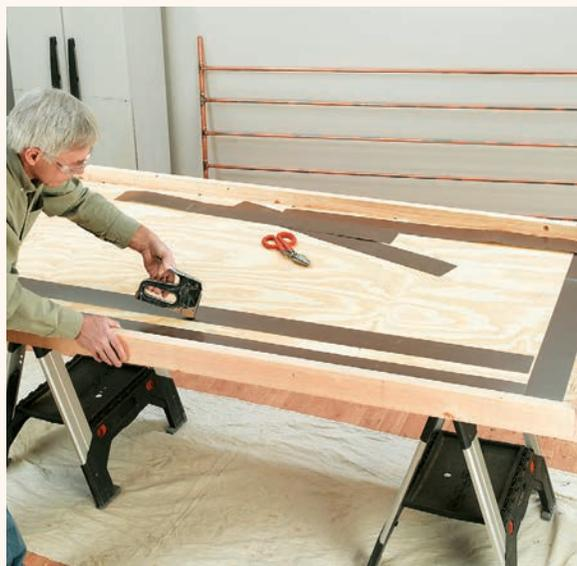
**9** Mark the manifold locations on the plywood, then cut 4"-wide pieces of aluminum flashing and staple them so they are centered under each length of copper. These will help transfer the heat to the copper pipes. Use stainless-steel staples.
