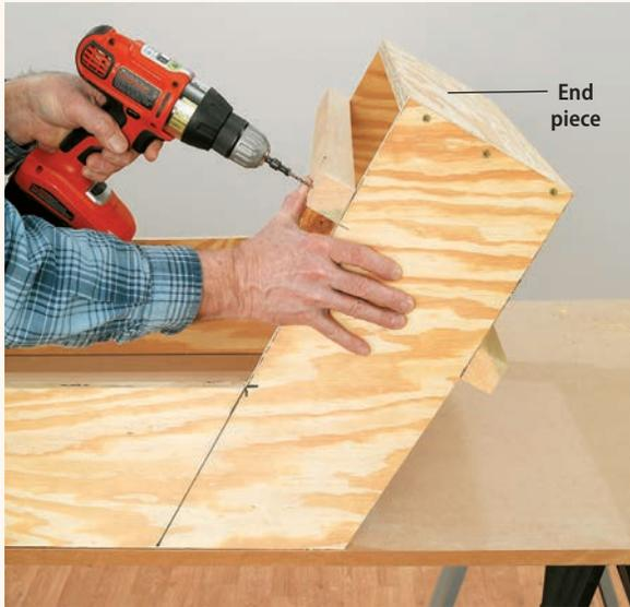
**3** Measure the distance between the stop moldings holding the window sash in, then subtract 1½" to get the length of the end pieces, which fit inside the side pieces. Pre-drill and screw the end pieces in place, then fasten 2 × 2s across the frame at the sash and sill locations.
