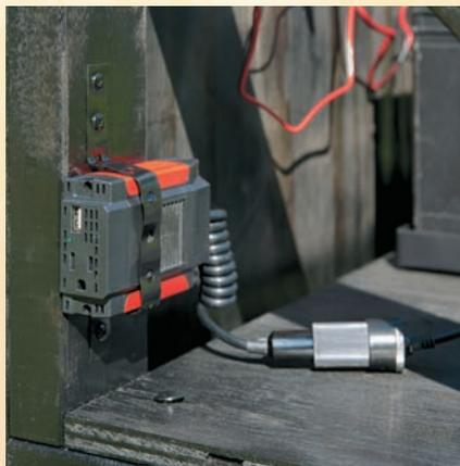
The circuit for a simple solar charging station is fairly basic. The electrical charge comes from the module, through an inline fuse and enters the charge controller. The charge controller is connected to the terminals of a deep-cycle, 12-volt battery. A power lead from a cigarette-lighter style DC plug goes to the output terminal on the battery. An AC inverter containing an AC plug and a USB port is plugged into the DC plug.
