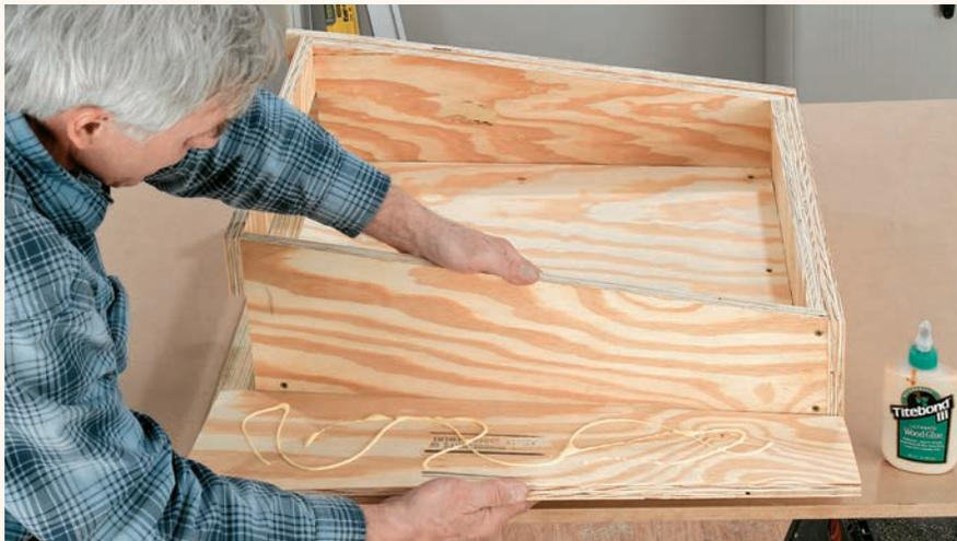
**4** Glue and screw the remaining front and side pieces on, using clamps to hold them together as you predrill and screw. Use 1¼" screws to laminate the pieces together and 2" screws to join the corners.
