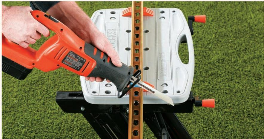
**3** Cut two additional pieces of strut to 4" less than the length of the expandable brace. Cut the expandable brace in half, then bolt both halves to the long center leg with four bolts. To expand the brace to the fall or winter position, just remove the bolts on one side, push the frame up, and then bolt the pieces back together. *NOTE: Solar collectors usually stay in a fixed position year round, while PV panels benefit from being moved to summer and winter positions.*
