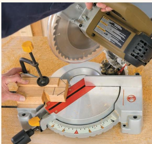
**3** Create the octagonal center block by cutting a 3" square of scrap 2x lumber ( $\frac{1}{2}$ " thick). Mark the center point by drawing diagonals, then draw a horizontal-vertical axis, as with the plywood base. Make a mark  $\frac{5}{8}$ " to both sides of the axis lines, then connect these marks to draw an octagon. Cut off the four triangular corners along these lines. Drill a  $\frac{5}{16}$ " hole through the center point to complete the block.
