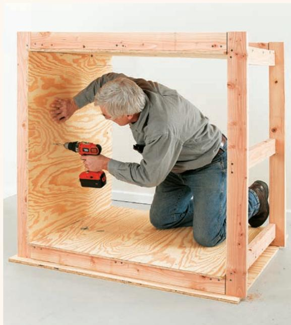
**4** Turn the box on its side. Fasten the plywood sides in place on the long walls, taking care to align corners and edges. Check the box for square as you assemble it.
