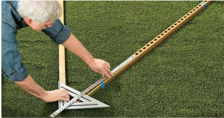
**2** Cut the pieces to length. Cut the cross supports to match the width of the solar collector or the length between mounting points on the PV panels.
