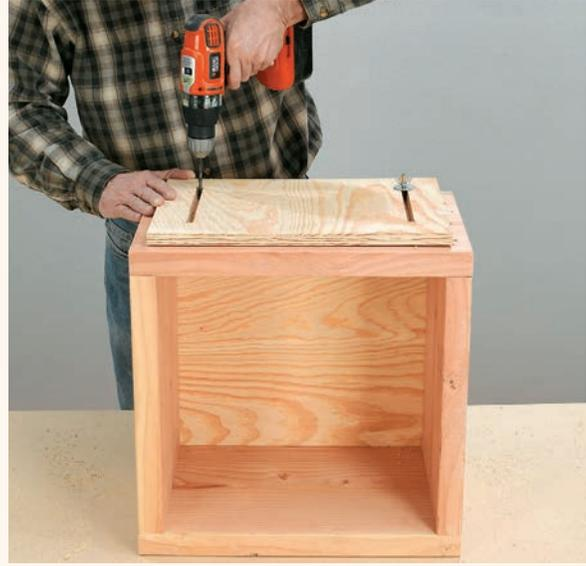
**8** Screw the base and the plywood bottom together. Set the adjustable leg against one side of the base, then drill guide holes and install the hanger bolts so they will align with the slots. The centers of the bolts should be at the same height: roughly 2½" up from the bottom of the box. Use large fender washers and wingnuts to lock the adjustable leg in position.
