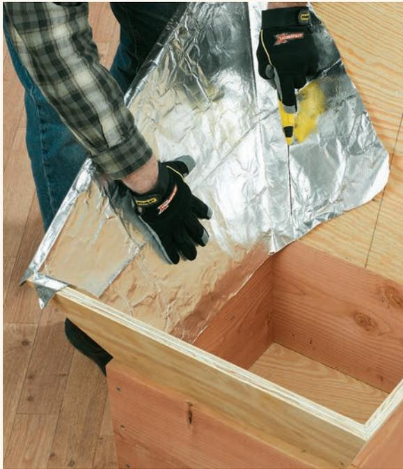
**10** Cut pieces of reflective sheeting to fit the sides of the reflector as well as the base. You can use heavy-duty aluminum foil, but for a sturdier option try solar foil (see Resources, page 186). The product seen here is essentially polyethylene tarp material with a reflective aluminum surface. Make sure to cut the pieces large enough so they overlap the edges and can be easily attached.
