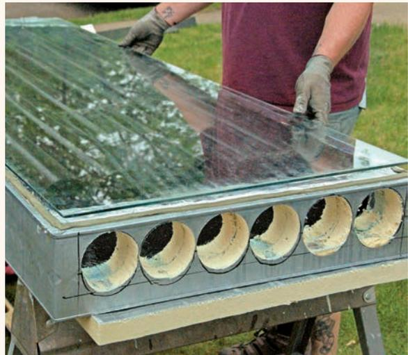
**12** Affix the glass top. First, double-check that all openings in the panel are adequately sealed and insulated. Then, line the tops of the steel stud frame with foam closed-cell gasket tape. Carefully position the glass on top of the gasket tape, lined up 1/2" from the outside of the frame on all sides. Then, position foam closed-cell gasket tape around the perimeter of the top of the glass panel.
