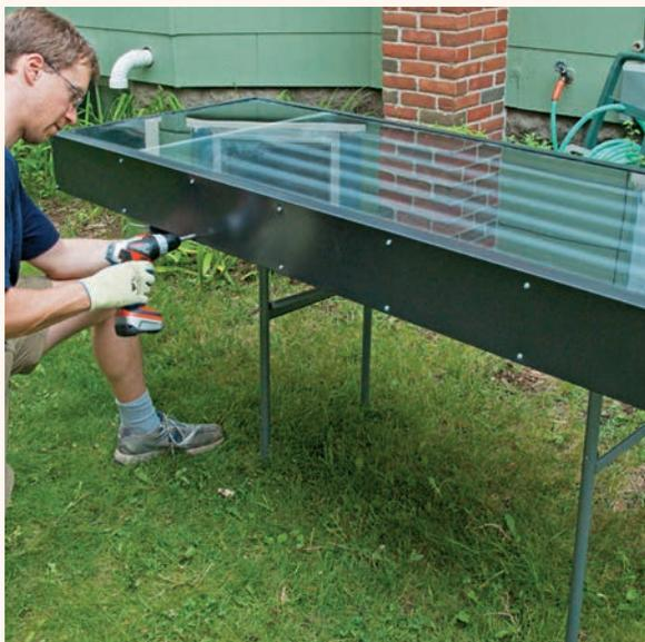
**13** Attach the casing. Work with a local metal shop to bend metal flashing that will wrap your panel box. Attach it around the perimeter of the panel with sheet-metal screws with rubber washer heads. *TIP: Be careful when working around the plenum ductwork. If you set the unit down on its back side, you will force the plenum up and break the seal around the opening.*
