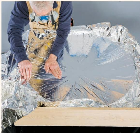
**10** Spray the dish surface with spray adhesive, then carefully lay a sheet of Mylar over the dish. Smooth the center area down, then work outward, spraying and smoothing as you go. Your goal is the smoothest possible reflective surface. Trim away the excess Mylar.
