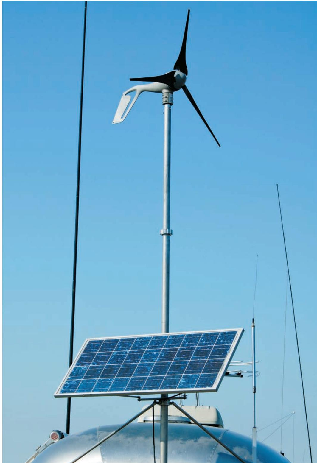
Lower-profile rigid mounts are designed for secure permanent mounting of modules. Some, such as the one above, are intended to be attached only when the vehicle is parked, and they can be combined with other power sources (even alternative sources such as wind).
