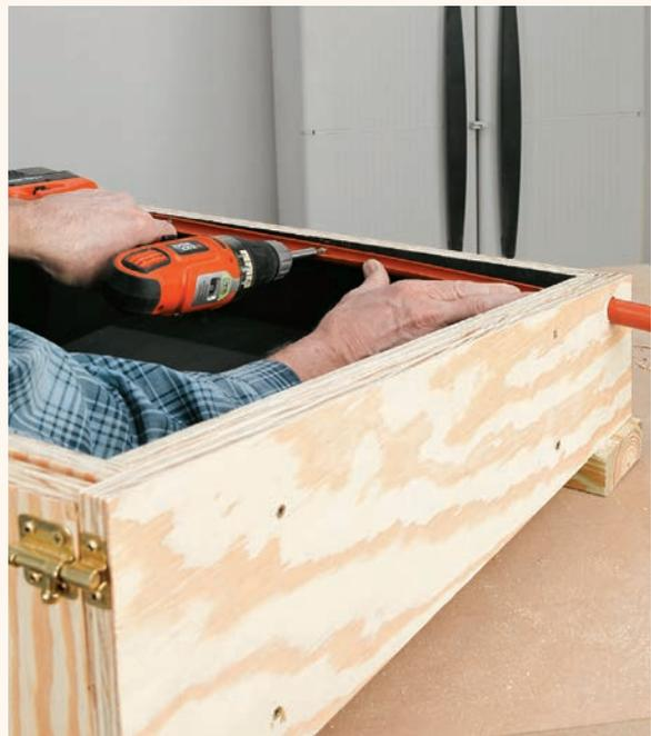
**10** Drill three  $\frac{1}{8}$ " holes in the side of the PEX for screws, then insert the PEX through the hole. Butt it tight against the other side, then screw it in place, sloping it about  $\frac{1}{4}$ ".
