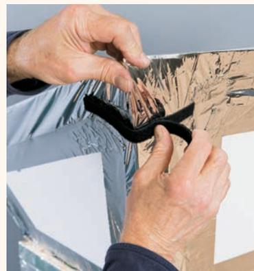
**6** Reposition the reflector panels on the oven box and align their edges at the corners. Cut 4"-long strips of hook-and-loop tape and apply one set of strips to secure the two adjacent panels together at each corner, about  $\frac{2}{3}$  of the distance up from the oven box. Apply the strips at an angle so they remain flat. Separate the strips and remove the panels for the next step.
