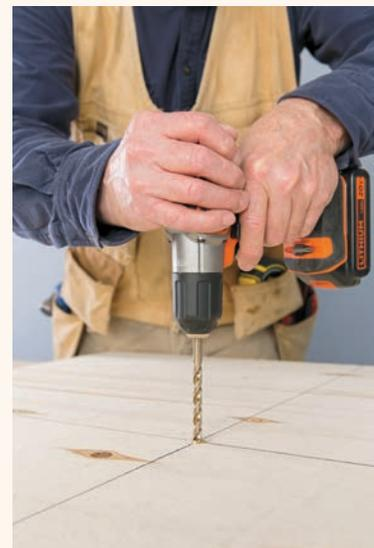
**2** Flip the plywood base over and draw horizontal and vertical axis lines on the backside. (You will use these lines later to position the leg assembly.) Drill a  $\frac{5}{16}$ " hole through the center point of the plywood base for installing the threaded guide rod later.
