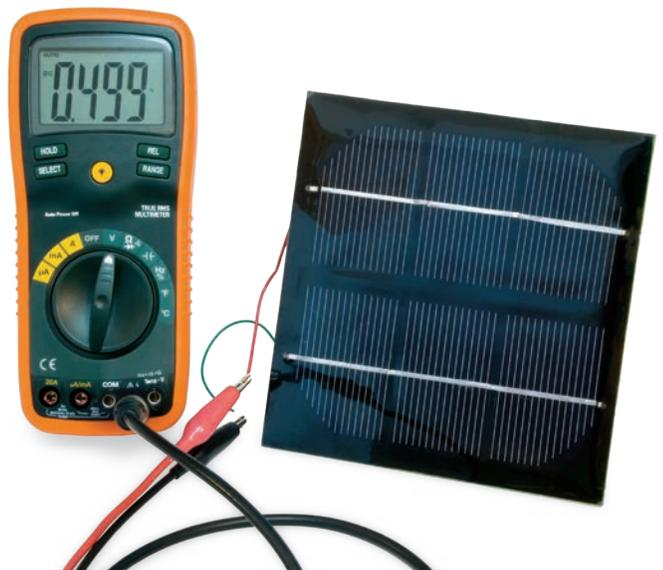
A multimeter is a good diagnostic tool for checking a photovoltaic module to ensure it is working properly. It also allows you to check the power generated at different angles and locations.
