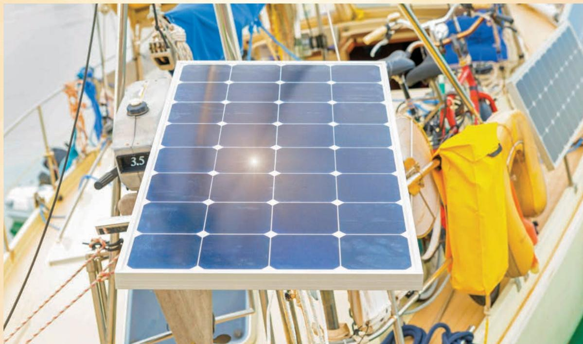
Adjustable mounts are available for sizable rigid modules as well as small portable panels. Mounts that rotate and tilt (or use ball joints for infinite adjustment) are the best for maximizing capture throughout the day.
