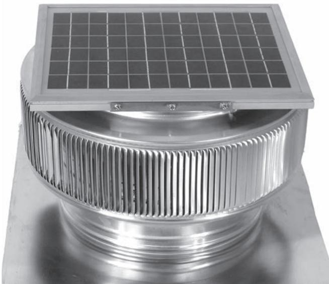
A solar-powered roof vent fan draws hot air from the attic during the day when the sun is out—the time when the attic is hottest. This type of fan generally does not include a battery, and is powered directly by the solar module (although some manufacturers offer models with backup wind or AC power).
