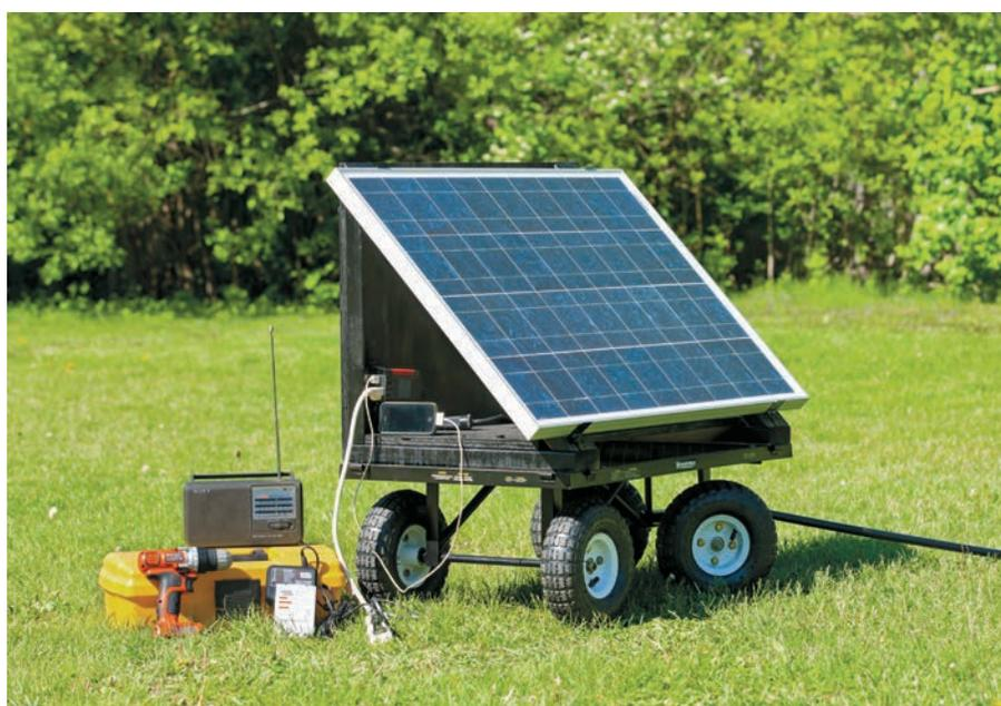
12-volt off-grid power systems are ideal for DIYers getting into solar electricity. Virtually the same system can supply permanent power to a shed or cabin, RV, camper, or boat to provide “house” power without help from an engine or generator (top), or be mounted on a wagon or trailer for portable power (bottom).
