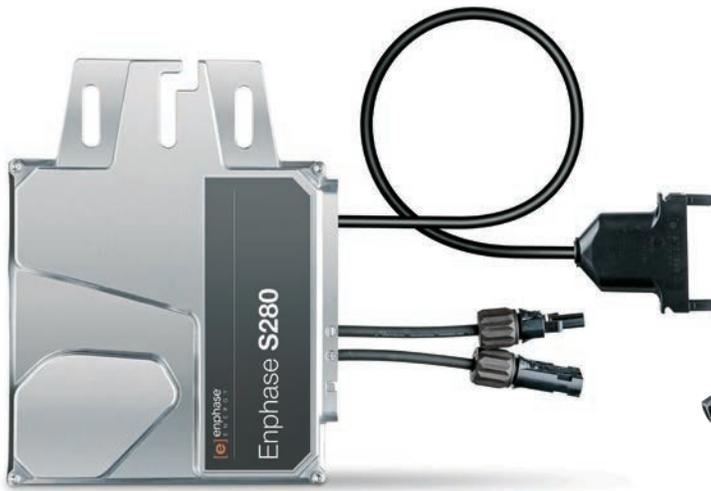
Micro-inverters are installed onto the module or the module mounting rack, then are connected to a cable (called a trunk cable) to form a branch circuit. A PV array may have one or more branch circuits, and each is joined to a junction box mounted to the module racking. *Enphase*
