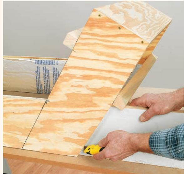
**4** Line the sides and ends with 1" polyisocyanurate insulation. Leave the foil side facing into the box and glue the insulation in place with construction adhesive. Wrap the exposed upper edges with aluminum foil tape to protect the insulation from UV rays. Cut the insulation ¼" narrower than the plywood sides so that the bottom piece of ¼" plywood will fit in between the sides.
