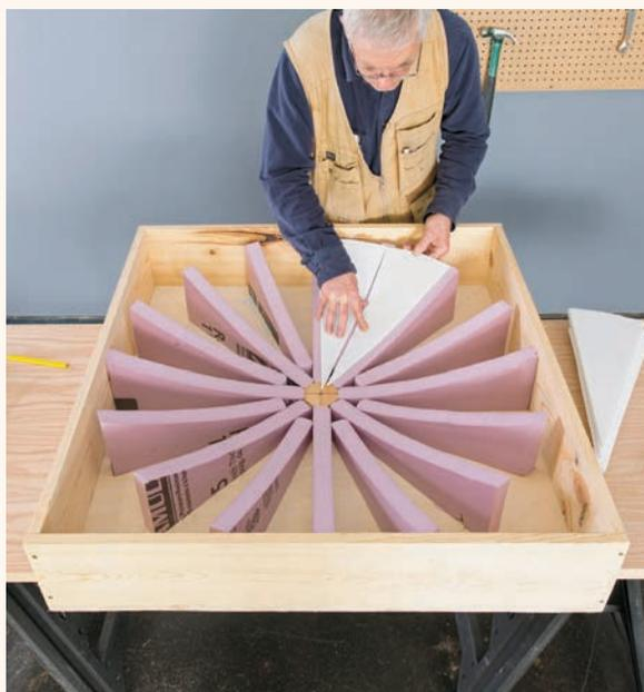
**8** Draw a panel template onto poster board as shown. It is a conical shape with  $18\frac{1}{2}$ " sides and a 7"-wide base. Cut out the panel template, then test fit it on several pairs of ribs, centering the panel on both ribs. Trim the template as needed for a good fit.
