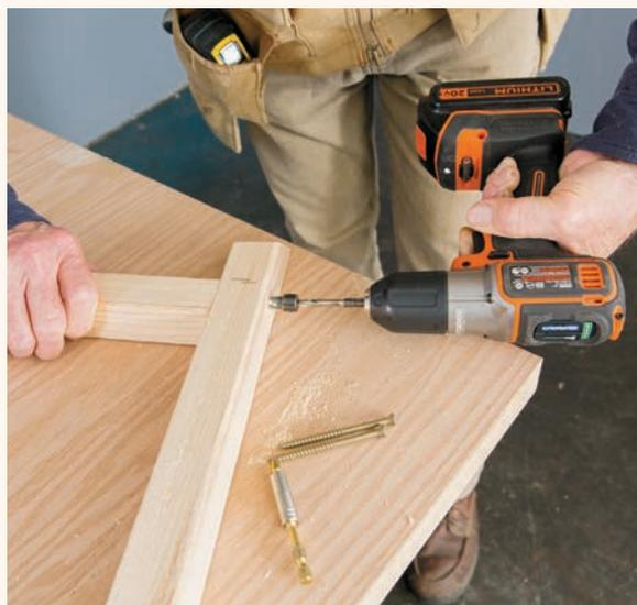
**12** Construct the leg assembly by cutting two 2" x 2" legs to length at 22", mitering the top ends at 45°. Cut two cross pieces at 17". Position the cross pieces between the legs, 3" from the ends of the legs. Drill countersunk pilot holes and join the pieces with two screws.
