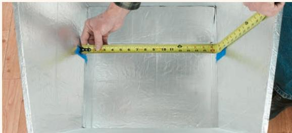
**12** Take measurements to double-check the glass lid size. Ideally, the lid will fit in so it comes to rest about 1" above the top opening of the box. As shown here, a  $\frac{1}{4} \times 17 \times 17$ " piece of tempered glass fits just right. Be sure to order glass with polished edges. You can also just use a clear plastic oven bag instead of the glass. Either will trap heat and speed up the cooking.
