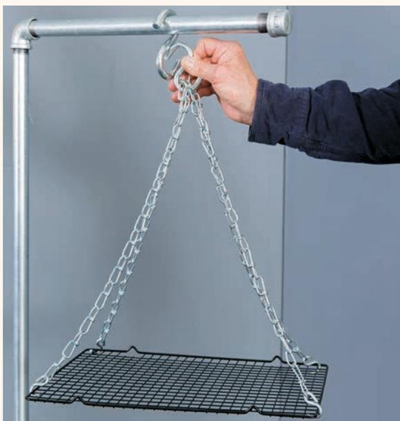
**15** Cut a 14" square of expanded metal using a jigsaw and metal-cutting blade. Use small S-hooks and four 16" lengths of chain to hang the metal square from a single S-hook in the center, then hang the assembly to the large S-hook on the stand with a 12" length of chain. *TIP: You can substitute a heavy-duty wire cooling rack for the expanded metal. Choose a size of rack that you won't have to cut down.*
