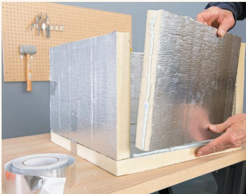
**1** Build the box by cutting two pieces of insulation board to size at  $12 \times 19$ " and two pieces at  $12 \times 16$ " for the four sides, using a utility knife and a yardstick. Cut one piece at  $19 \times 19$ " for the bottom. Glue the sides together over the bottom with foamboard adhesive to form a  $19$ " square. Tape the pieces in place, and let the adhesive cure as directed. *NOTE: Any insulation board you use must be rated for temperatures higher than  $450^\circ\text{F}$ .*
