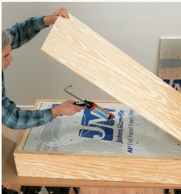
**7** Turn the box over, add the 1" insulation to the bottom of the box, then cover it with the  $\frac{1}{4}$ " plywood. Glue the plywood to the insulation and screw it to the  $1 \times 3$  nailer with  $2\frac{1}{4}$ " screws.
