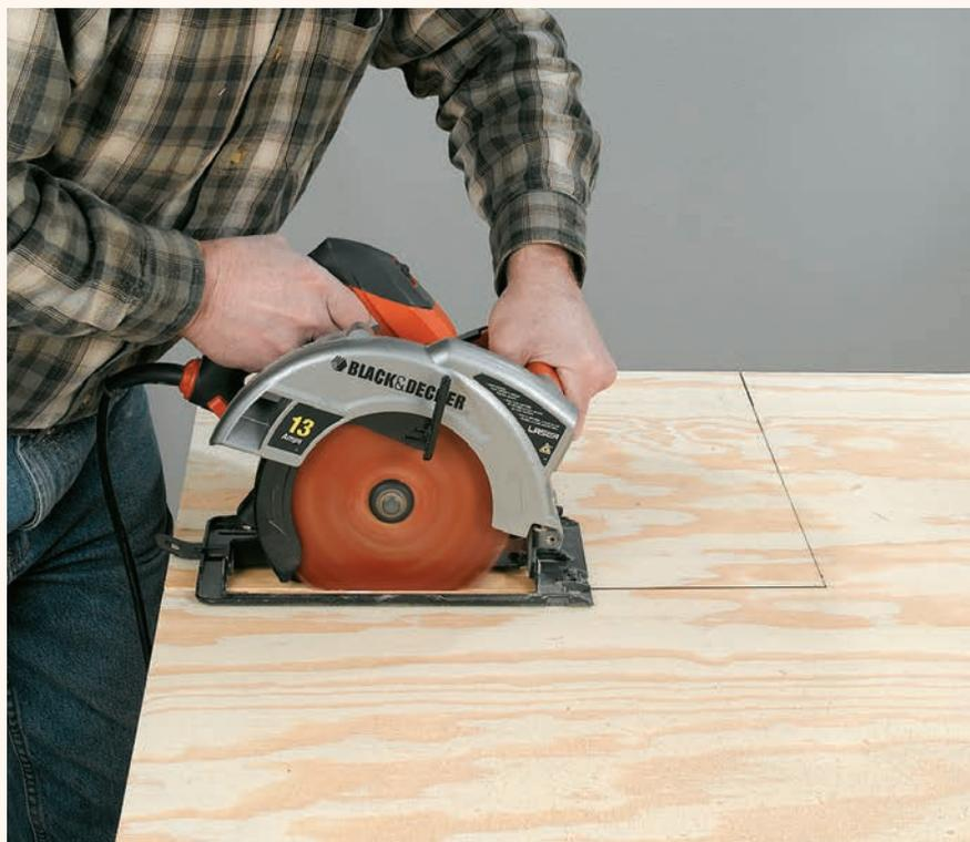
**2** Lay a 4 × 8' sheet of plywood on the worksurface with the better side facing up. Select a good grade of ¾" plywood (we used BC) or you're likely to have issues with parts warping, and you'll find it difficult to drive screws into the edge grain of the plywood. Mark and cut the 19 × 19" bottom piece first. Rest the full sheet of plywood on a couple of old 2 × 4s—you can cut through them as you make your cuts without any need to move them out of the way.
