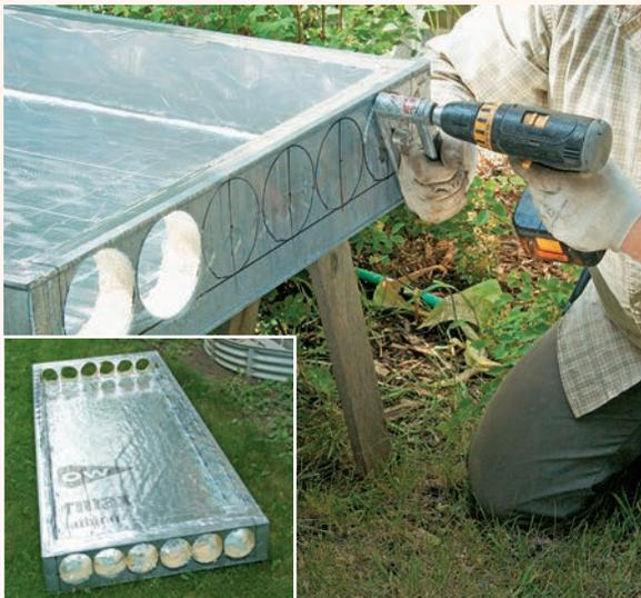
**7** Create inlet and outlet holes in the walls with a hole saw or circle cutter. The number and location of the ductwork holes depends on where each panel fits into the overall array (presuming you are making and installing multiple panels). The first and last panels in the series will each have one end wall that is uncut, while intermediate panels will have duct holes on each end wall (inset).
