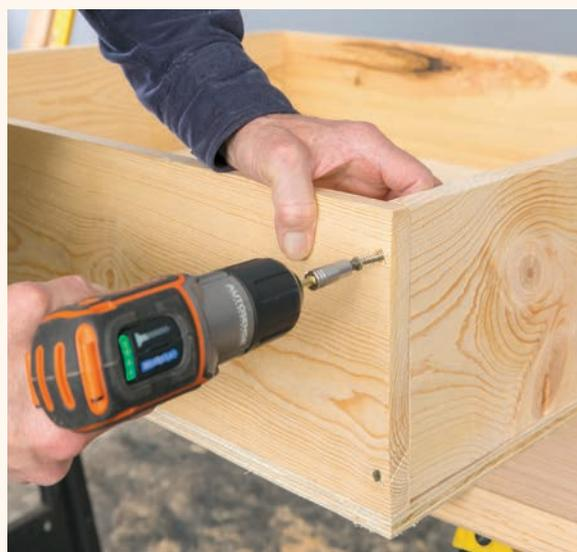
**4** Cut two pieces of  $1 \times 8'$  to length at  $36"$  and two pieces at  $37\frac{1}{2}"$ . Apply construction adhesive to the bottom edges, and glue the boards along the edges of the top face of the plywood base, so the longer pieces cover the ends of the shorter pieces. Drill pilot holes, and screw the boards together at the corners, using  $1\frac{1}{2}"$  screws. Also fasten the boards with screws driven through the bottom of the base.
