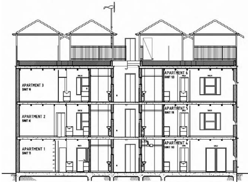
4.10 Section of the apartment building
